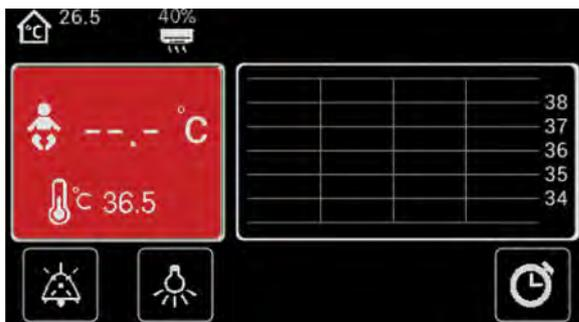
3.12 Probe Failure alarm.
