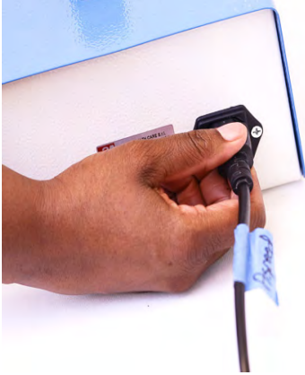
7.1 Check that power cable is securely attached.
